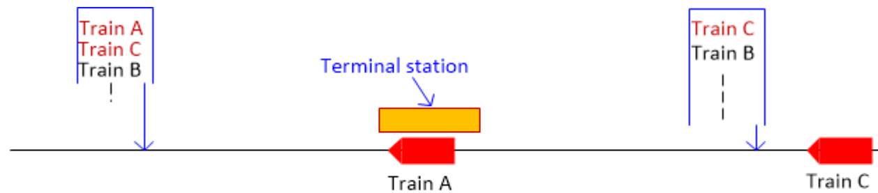
Figure 20: Intermediate terminal station
