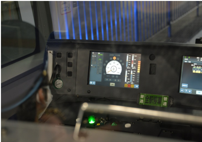
Figure 13: Tokyo monorail cab showing VDU style speedometer including indication of authorised speed.
