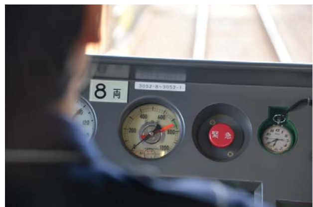
Figure 12: Tokyo Keikyu line cab showing electromechanical speedometer (part hidden by driver).
