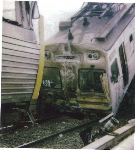
The catastrophic collapse of the Clyde car when the set crashed into the rear end of a Comeng train at Syndal station on 20 November 1989.
