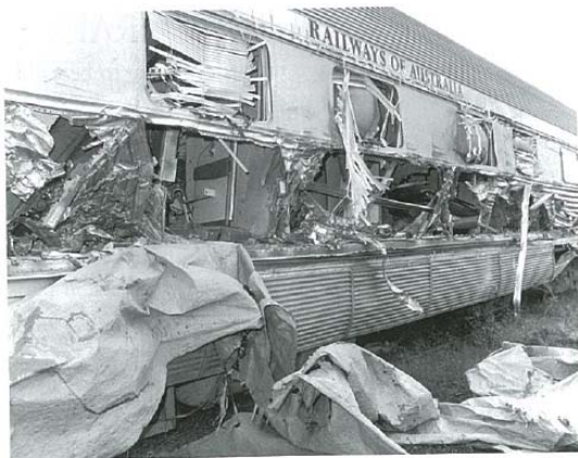
One of the Indian Pacific cars at Comeng Granville showing the extent of the damage when the train was sideswiped by a derailed goods train at Locksley during a trial run only five days before revenue service between Sydney and Perth was due to commence.
