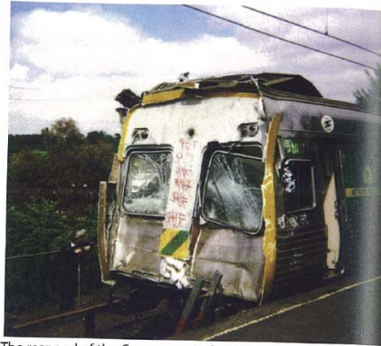
The rear end of the Comeng train following the collision. The damage was moderate and repairable.
